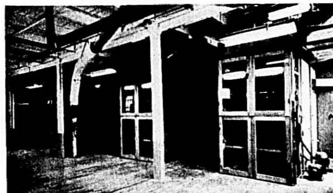
BATTERY of Hoskins continuous dryers for short-cut macaroni products—elbows, shells, and noodles. Variable drive (Reeves) permits wide speed changes for products with different wall thicknesses. Right: Schematic diagram shows control elements in section view. Mixed conditioned air enters chamber at bottom of dryer.
